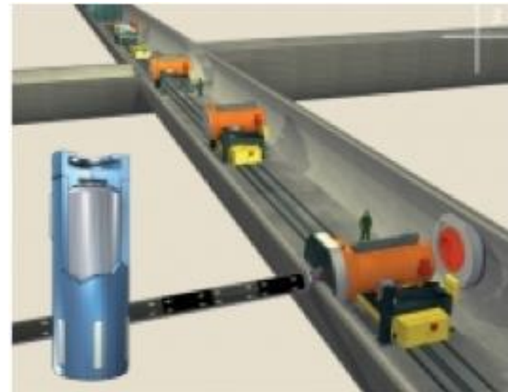
Before being emplaced in disposal cells, HL radioactive-waste packages are conditioned in disposal containers.
